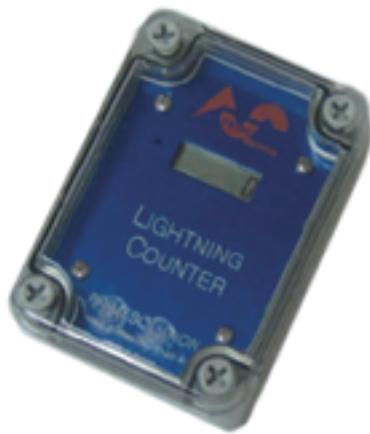
The ALC-100 is a lightning current counter that counts the number of current pulses occurring with lightning in the down conductor of a extra lighting protective system or the grounding conductor in a building. The ALC-100 would make it to be convenient for the LPS supervisor to manage the LPS actually. It is easy to install the ALC-100 without cutting the cables, and it also could be positioned without additional housing at outdoor atmosphere because it was designed to be waterproof.
